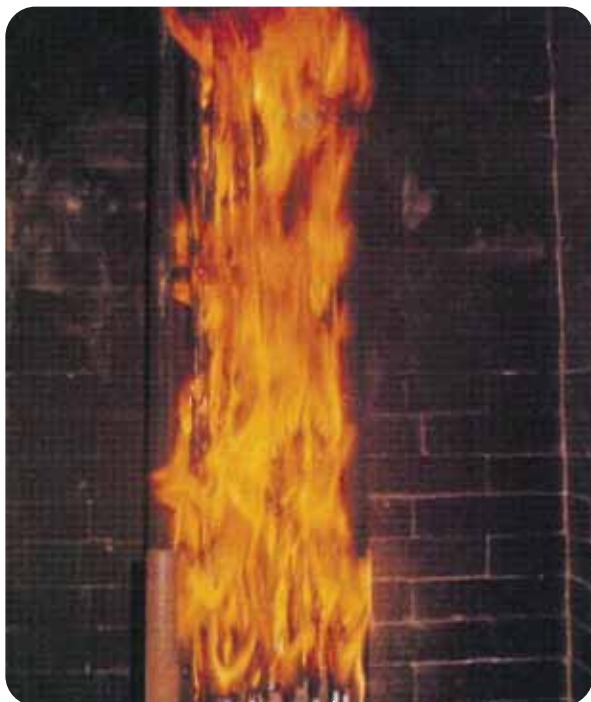
Standard PVC cable during flame conductivity test
