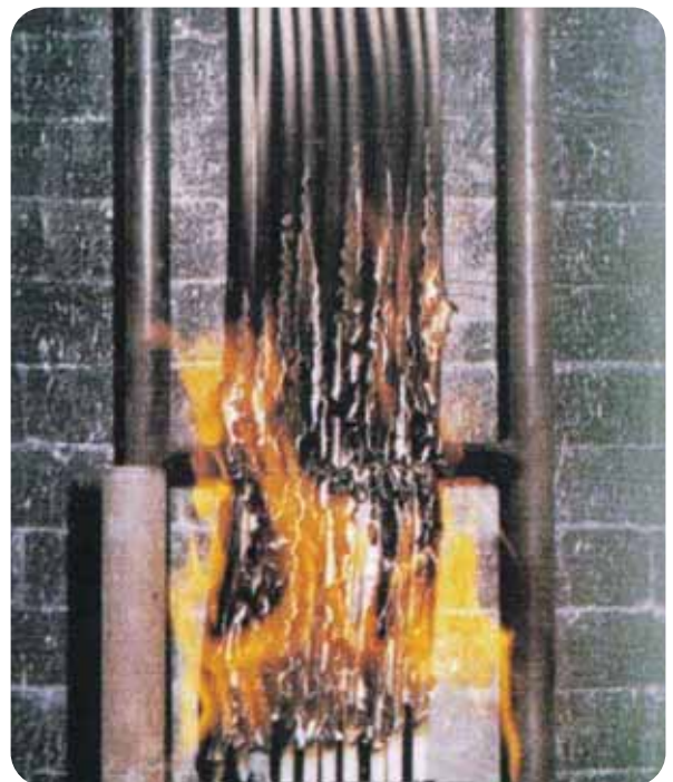
AFUMEX™ cable during flame conductivity test
